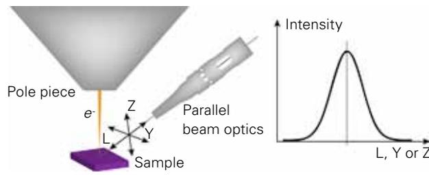
XSense can position the spectrometer optics along 3 axes for perfect automatic alignment.
