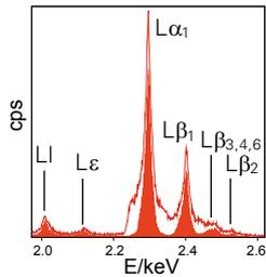
Molybdenum spectra obtained with standard (outline) and advanced optical system (solid).
